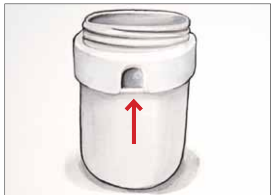
Lugs are located on each side of a centrifuge bucket
