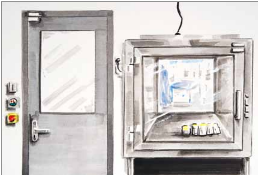
A pass-through box is an airlock for small items
