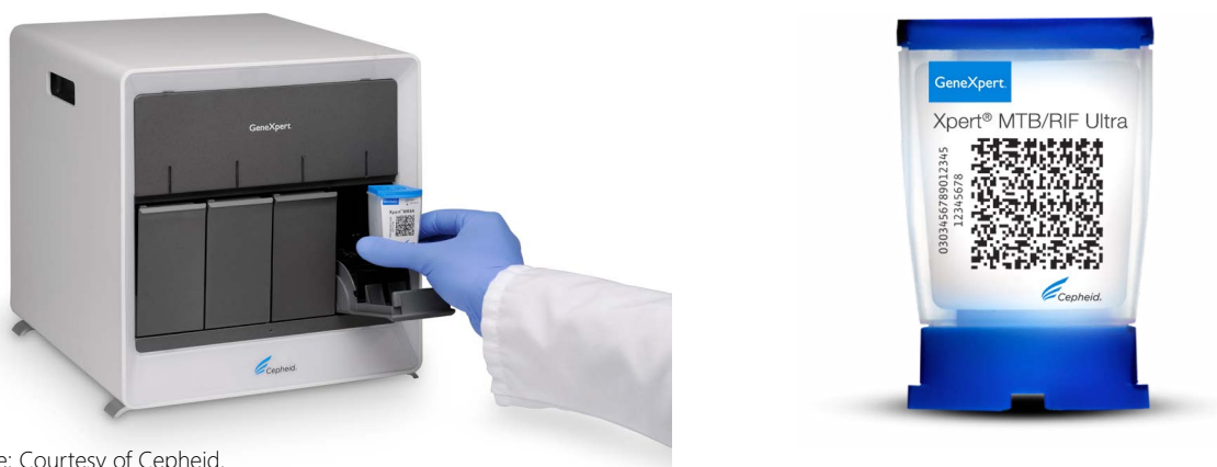
Fig. 1.1. The GeneXpert four-module instrument and the Xpert MTB/RIF test cartridge
