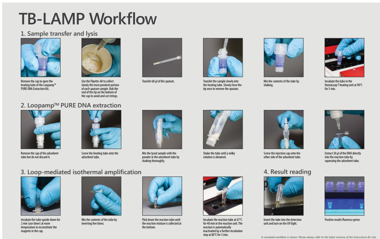
Fig. 2.2. Description of the workflow for TB-LAMP
